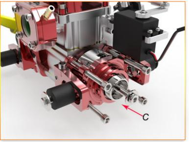
Match the clutch bell with front plate onto clutch shoe and tighten it with supplied M5x40 bolts and spacers, then secure the M6 center bolt and washer into crankshaft, the M6 bolt must be applied with loctite before tighten.
