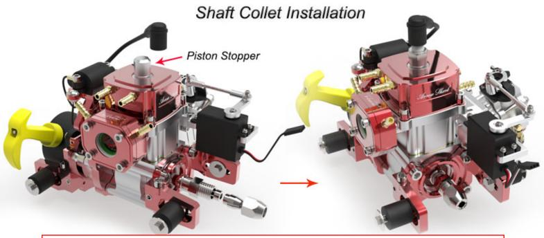
Screw the piston stopper into the spark plug hole, and install the shaft collet base on the crankshaft and tighten it with supplied M6x16 bolt, then insert the front adaptor into the base, screw the top cap down.
