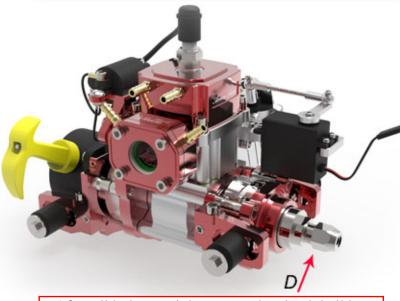
After all bolts are tighten, turn the clutch bell by finger to make sure it is spinning freely, then, screw in the front adaptor and install the insert and cap.
