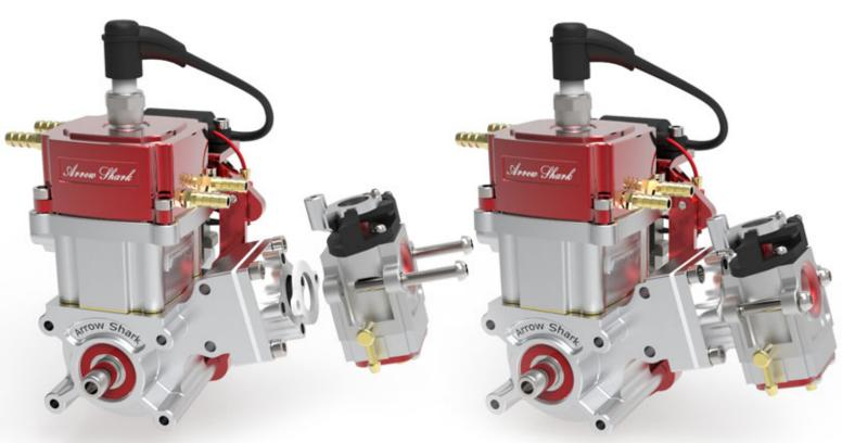
Insert the supplied M5x40 bolts via the supplied Teflon gasket and carburetor, and then tighten them to secure the M-39X carburetor to the billet reed valve.
