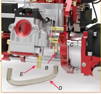
The X-30 marine engine comes with unique design of pop-off pressure for the incoming gas, there is a pulse nipple has been installed on the M-39X carburetor with a pulse-line connection to the X-30 billet reed case for delivery the pressure from engine to M-39X for the most smooth and effective gas conveying.
