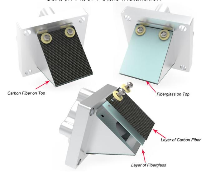
The reed valve petals in X-30 was custom compounded by high quality carbon fiber and fiberglass sheet in order to achieve optimum flapping tension control for the long lasting performance, the both side of the petal can be installed for the operation, when fiberglass side is damaged, just simply flip it over and use carbon fiber side till both sides damage, then replace a new one.
