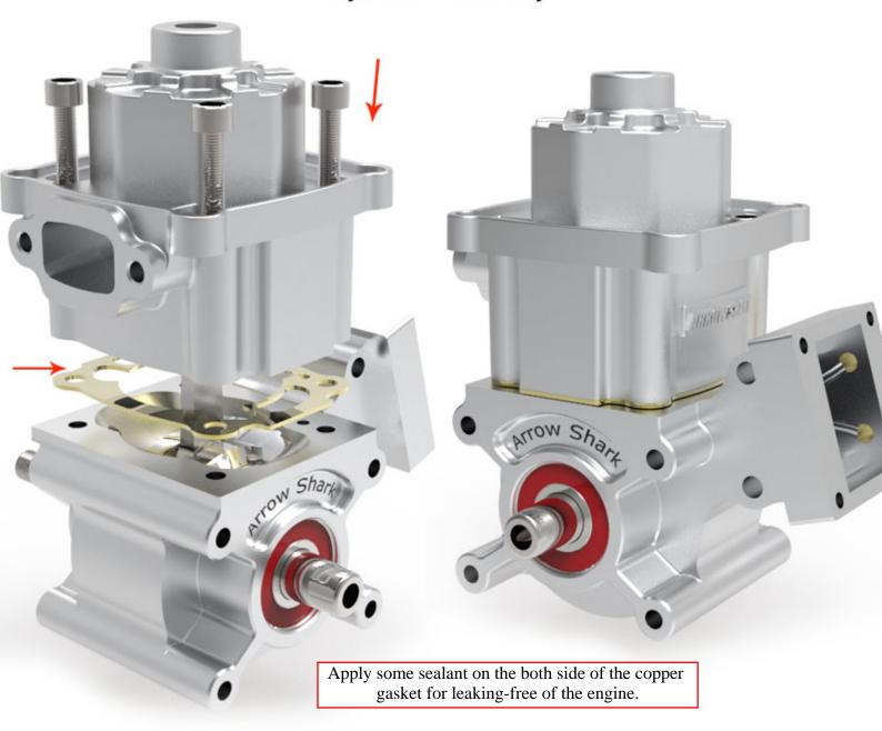
Use a small slotted screwdriver to fully adjust the piston ring into the cylinder, then screw down the bolts through the cylinder all the way into the crankcase. Tighten the bolts a little at a time in turn until they are fully secure. All bolts must applied with mid strength loctite.
