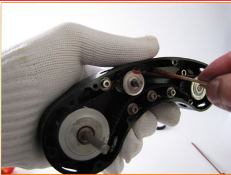
Install the main drive belt onto the wheels in the CNC belt housing and apply some grease on the back of the drive belt as shown in the picture above.
