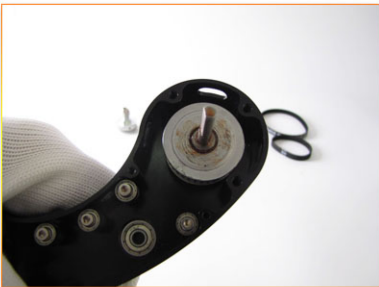
Install the one way bearing wheel into the CNC belt housing. (Please make sure the belt wheel has correct side up, when you turn the one way bearing shaft forward, the wheel must spin with the shaft.)
