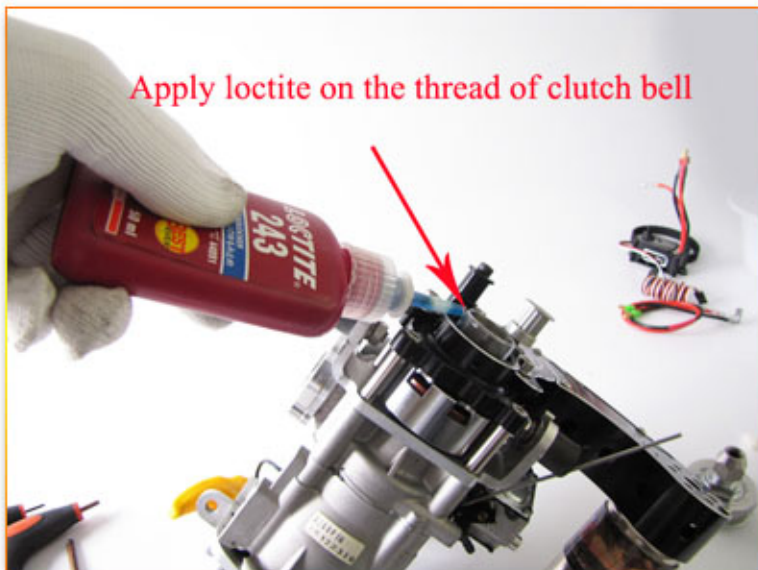
Apply some loctite on the front thread of the clutch bell. ( Note: this is very important, without the loctite, the main wheel assembly will get loose out when engine runs, when you try to unscrew the main wheel assembly out of the clutch, you have to heat the thread area first before screw it out)
