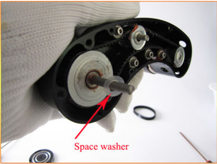
Install the plastic spacer onto the one way bearing shaft as picture shown above. Install the front drive cover onto the CNC belt housing and tighten it with M4x12 bolts and CNC washers.
