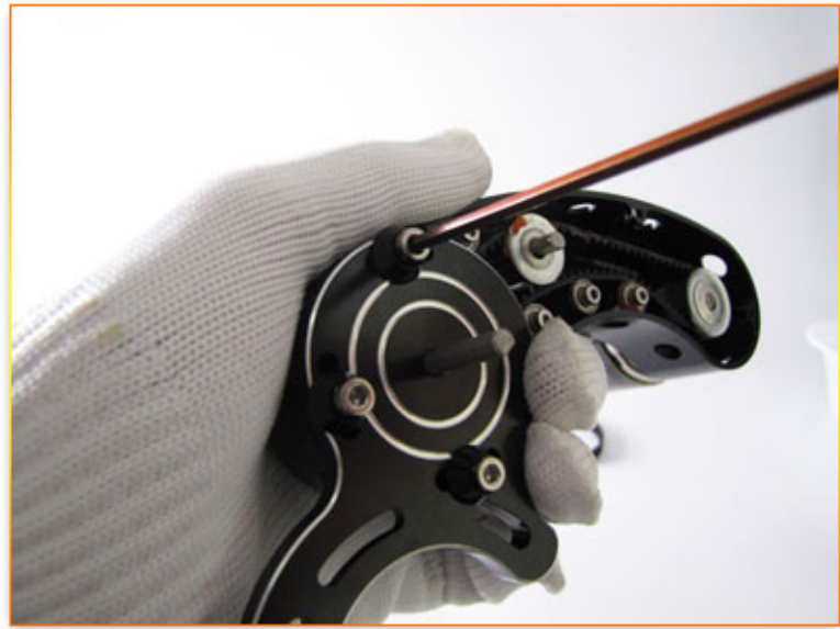
Install the plastic spacer onto the one way bearing shaft as picture shown above. Install the front drive cover onto the CNC belt housing and tighten it with M4x12 bolts and CNC washers.
