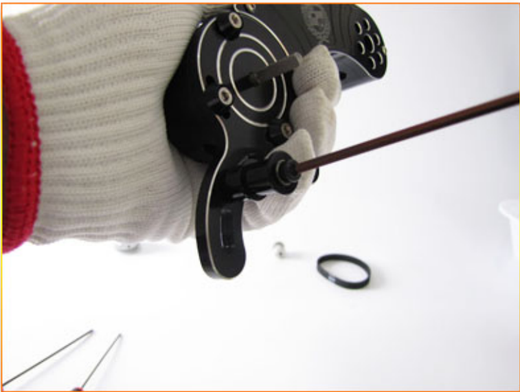
Screw the transfer wheel assembly into the M4 nut from front of the drive cover, but, not to tighten it at this moment.
