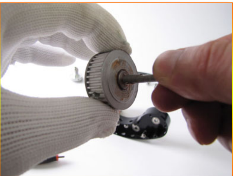
Insert the one way bearing shaft into the bearing, and rotate it for few rounds in order to make the grease hiding between needles inside the one way bearing.
