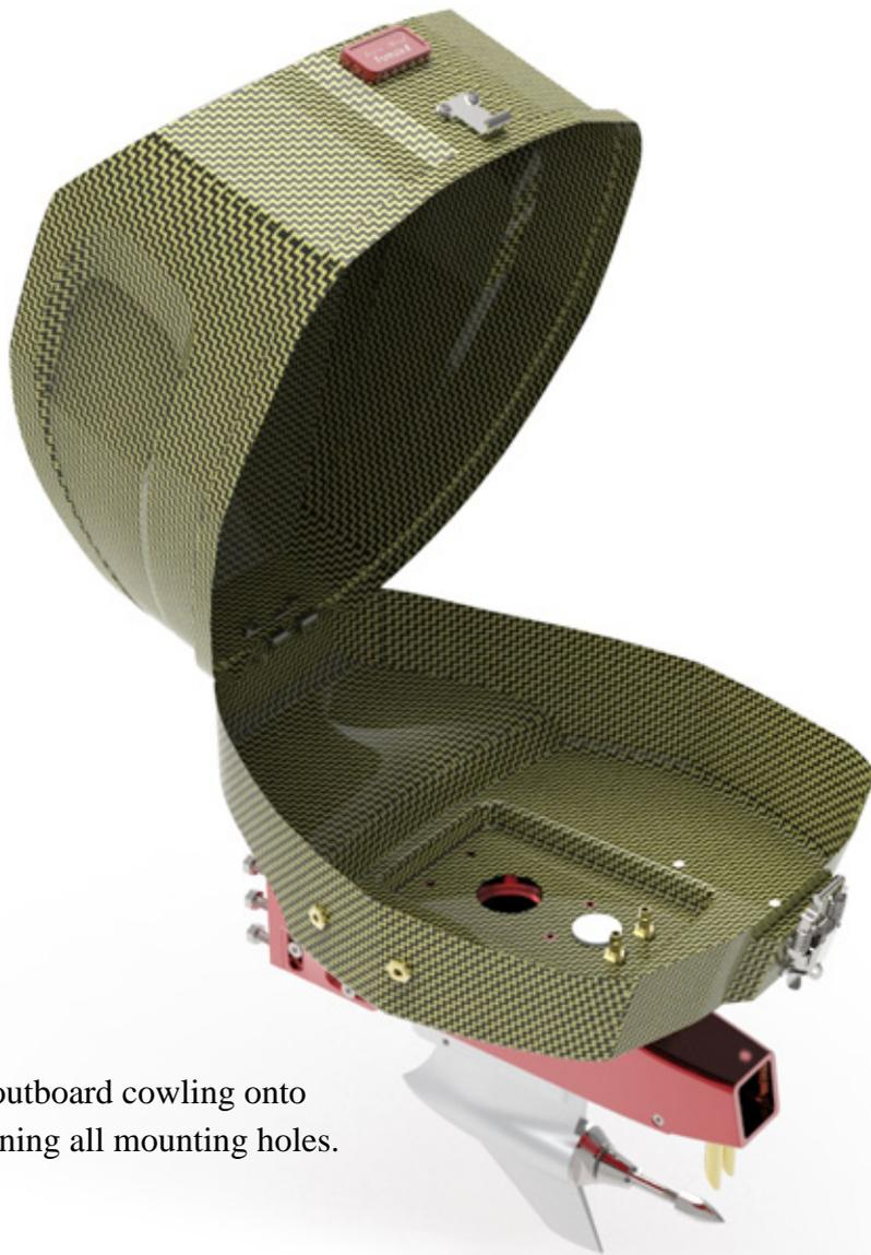
Match the outboard cowling onto Drive, Aligning all mounting holes.
