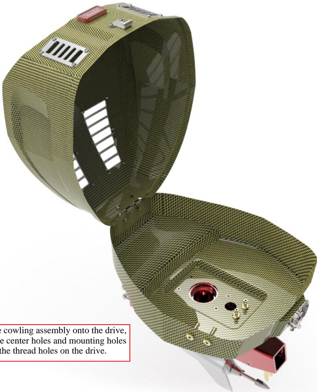
Place the cowling assembly onto the drive, match the center holes and mounting holes to the thread holes on the drive.
