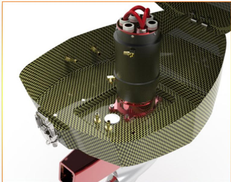
First, install the drive shaft into the coupling, then, insert the drive shaft along with electric motor assembly into the square input on the center barrel shaft, then tighten the bolts to secure the electric motor assembly onto drive.
