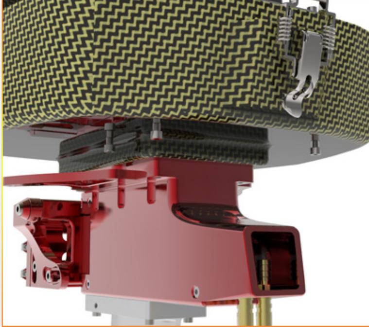
Install the ESC, LIPO battery and Mounting bracket assembly into the outboard cowling, and secure the bolts from the bottom of the cowling. then connect the wires between electric motor, ESC and LIPO battery.
