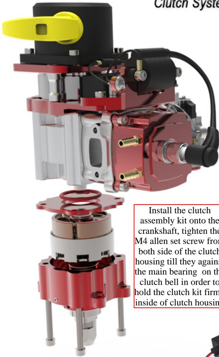
Install the clutch assembly kit onto the crankshaft, tighten the M4 allen set screw from both side of the clutch housing till they against the main bearing on the clutch bell in order to hold the clutch kit firmly inside of clutch housing.
