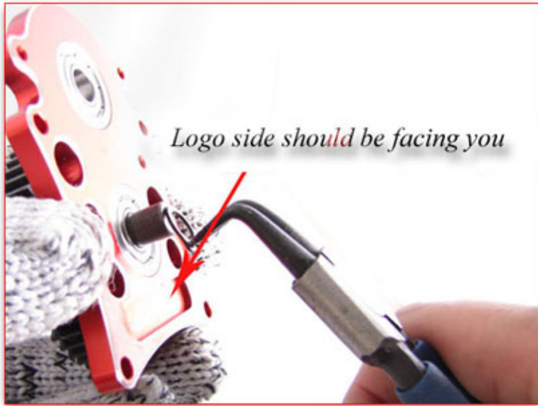
Insert the coupling shaft through the lower bearing on the CNC plate as shown above, and use a C-clip to hold the shaft in place. Note: When doing this, the Logo side should be facing you.
