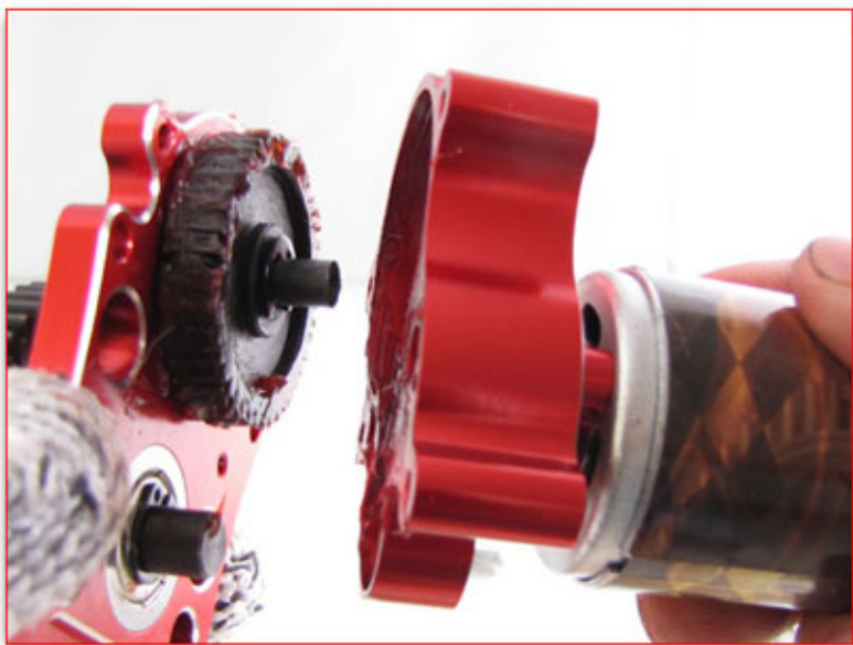
Match together the CNC plate and the gear box as shown above.
