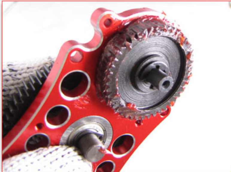
Apply some grease in the gap of each tooth on 35T gear as shown above.
