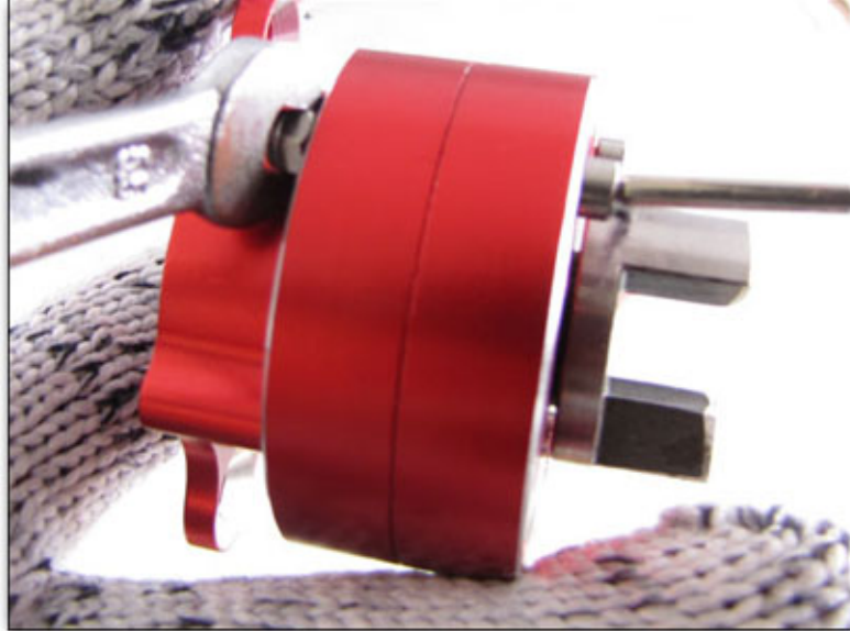
Tighten these two clutch box pieces with bolts and nuts.
