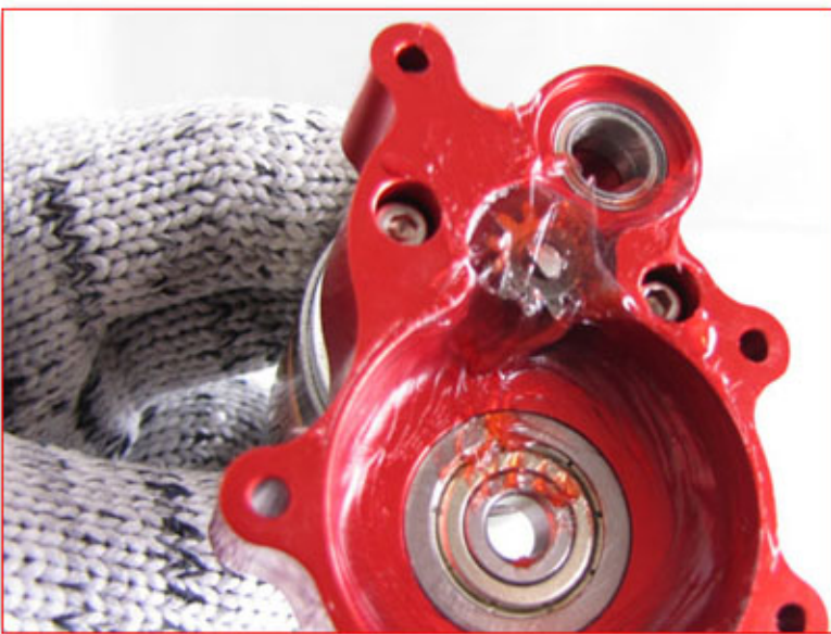
Apply some grease on the side of the gear box and electric motor gear.
