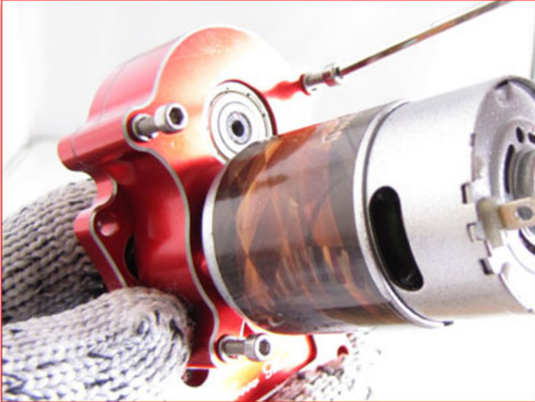
Use M3x25 bolts to hold the gear box firmly on the top of the CNC plate.
