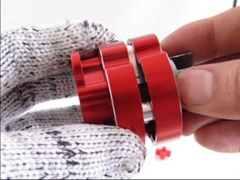
Assemble the upper and lower clutch boxes together - making sure the slot will match.
