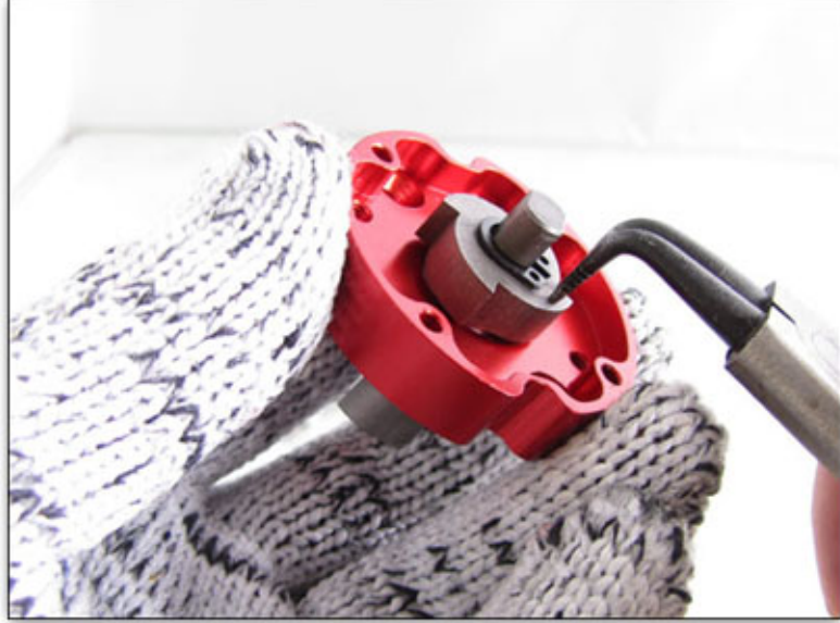
Apply the C-clip onto the shaft in order to hold the spinner in place.
