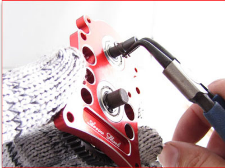
Use the C-clip to hold the gear shaft in place.
