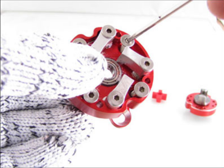
Install the upper clutch box assembly to the flywheel adaptor, and tighten it with four bolts.
