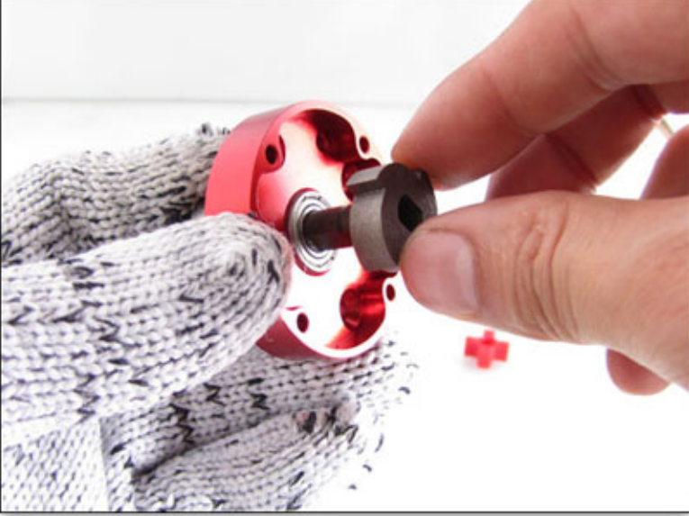
Insert the four leg spinner onto the coupling shaft.
