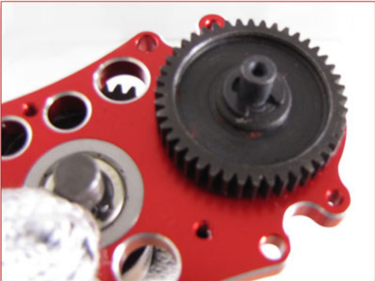
Insert the 35T gear onto the shaft on 13T gear shaft and use a C-clip to hold it in place.
