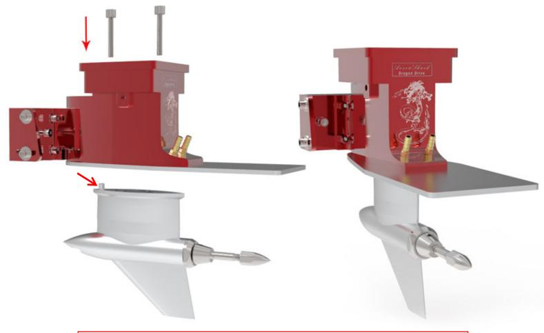
Now get both upper and lower assembly units ready for Connecting these two parts together and make sure the water intake nipple on the lower unit is properly aligned into the matching hole on the riding plate. Using two M5x25mm bolts, tighten these two parts together as shown in the above right picture.
